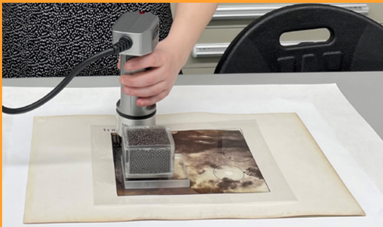
Colorimetry measurements in progress on an Alexander Henderson photograph, MP-1976.122.2.4.
